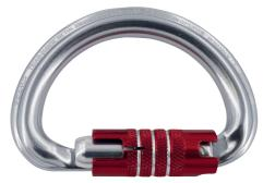
Automatic lock requires three actions to open: slide, twist and pull.
