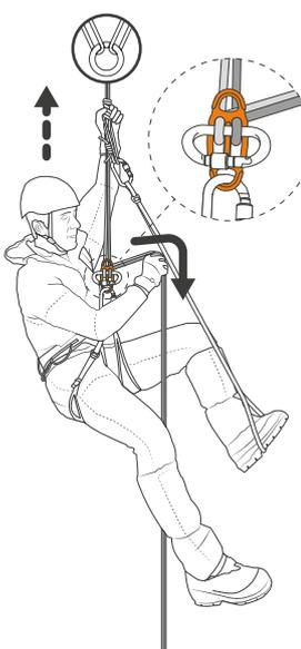
The diagram shows a person ascending a rope. A descender is attached to the rope, and a Prusik knot is used to pull the rope up. An inset shows a close-up of the Prusik knot being pulled over the descender.
