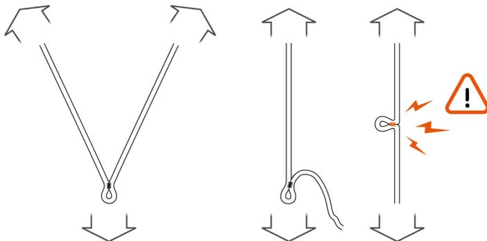
Poor positioning that prevents locking
