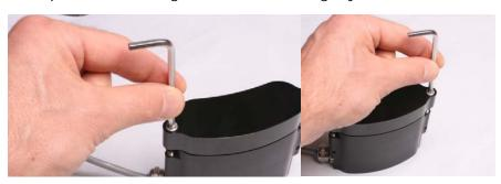
Next, tighten both screws **alternatively**. Tighten each screw by 90°, and then tighten the other one! This prevents the lid to be tilted, which could affect the waterproofness of the seal.
